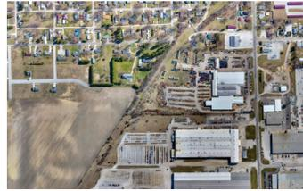
Orthomosaic maps are created by stitching multiple overlapping drone aerial images, via mapping software, into a single geometrically corrected or “orthorectified”
