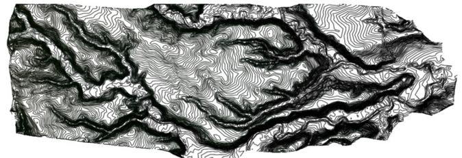
Millions of X,Y,Z data points are generated when a drone collects overlapping aerial images from a typical site. These data points allow for the creation of topographic maps with contour intervals as dense as 1 ft. Topographic maps created by drone aerial imagery provide the same relative and absolute accuracy as orthomosaic maps.
