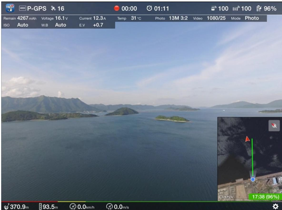
iPad Navigation Map and FPV live video can be displayed with P-in-P (above) or Side-by-Side (below) layout. Custom Telemetry can be shown in either Horizontal (above) or Vertical (below).
