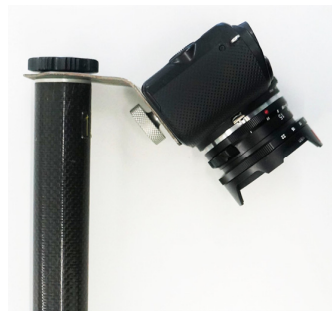
Figure 4. Camera holder for terrestrial photogrammetry.
