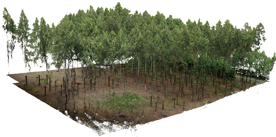
Figure 6. 3D view of point clouds from terrestrial and aerial photogrammetry.
