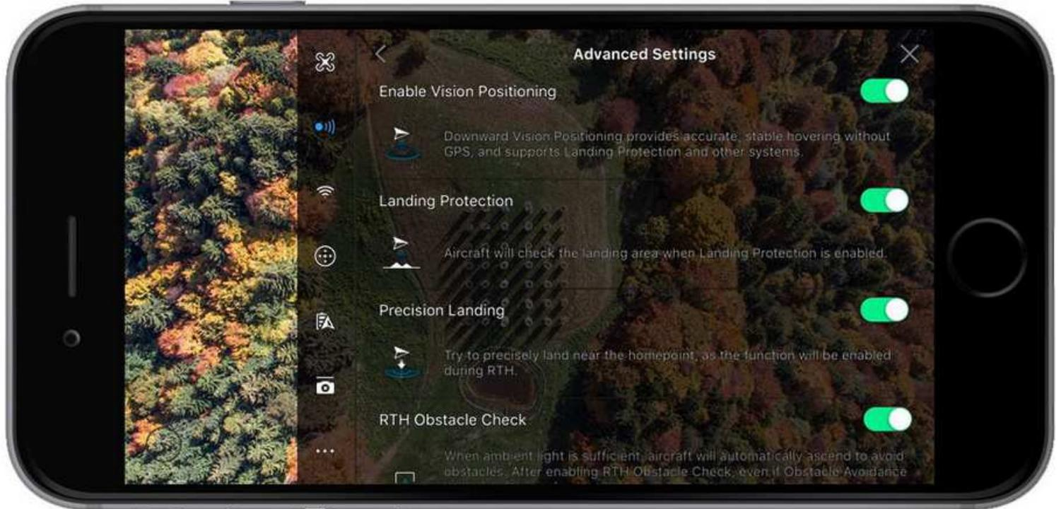
**Enabled Vision Positioning:** If this is toggled then the downwards sensors will be turned on which will help to keep the aircraft in a fixed position when hovering. When turned off your aircraft will drift when it hovers if the GPS signal is too weak.
