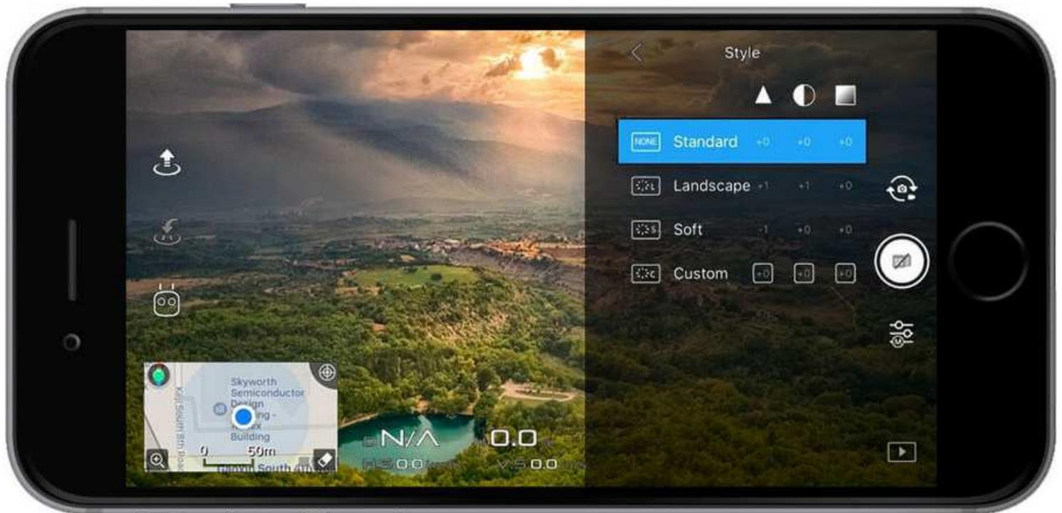
This is where you can configure the sharpness, contrast, and saturation of the images or videos that your drone's camera takes. (Triangle) Digital Sharpness this makes the picture sharper. (Circle) Contrast controls the strength of the lights and the darks in the picture. (Rectangle) Saturation of colors low saturation makes the photos look dull, and high saturation make the colors pop. These can be set in a range of -3 to +3.
