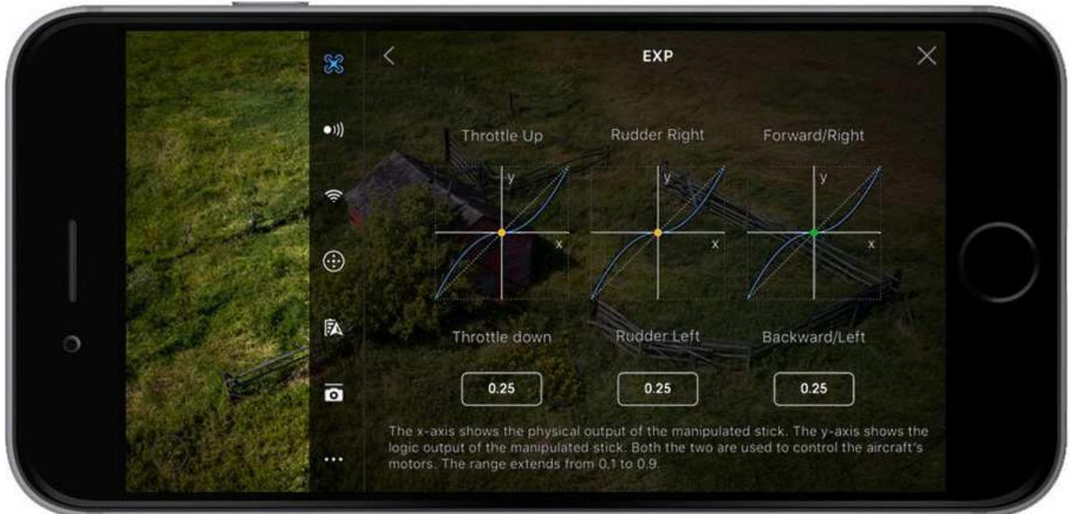
**EXP** values reflect the logical relationship between the control stick movements you make and the feedback from the aircraft. The X-axis represents how much the control stick is being pushed, and the Y-axis represents the amount that the aircraft responds based on the adjusted EXP value. **(Not available on Spark)**
