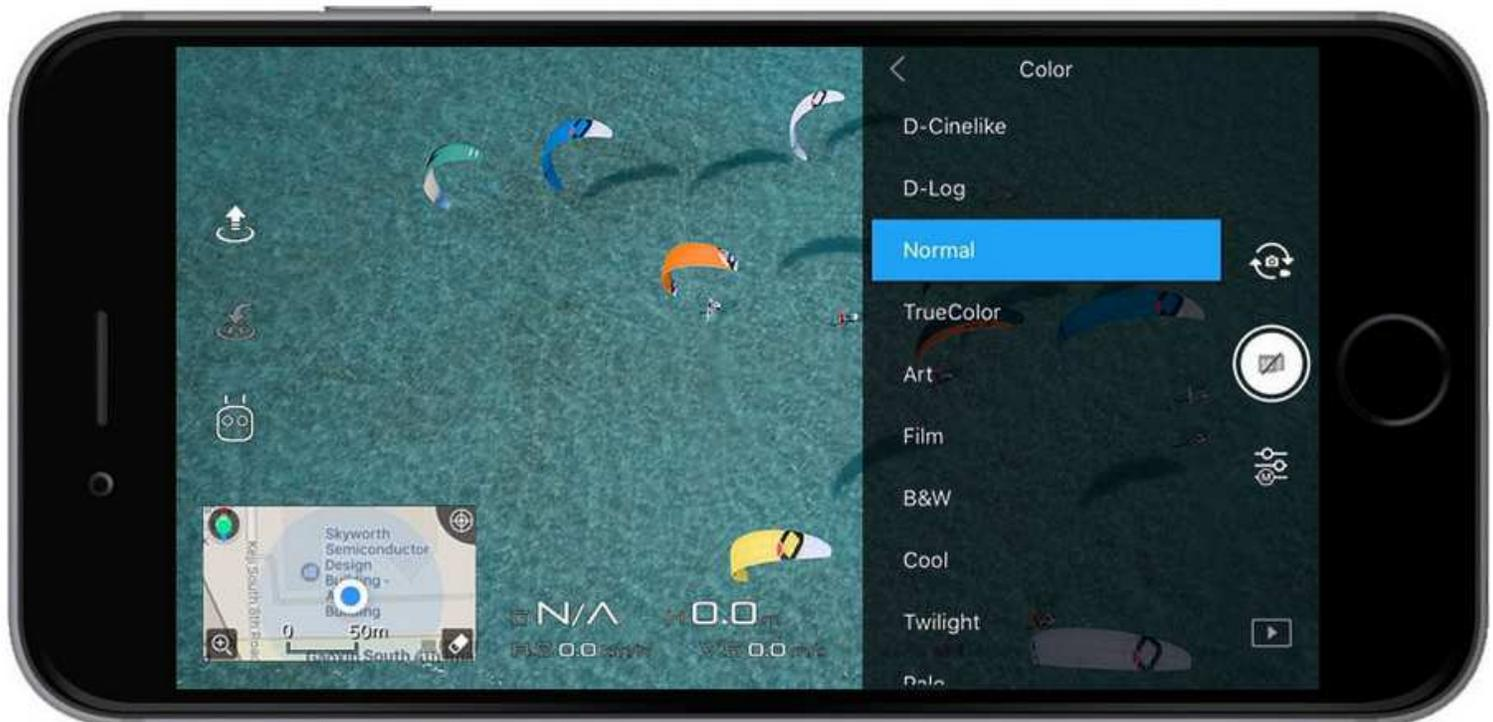
Here you can set the camera color profile. These settings affect the colors in your photo. D-Cineline and D-Log are both designed for taking photos that will be post-processed later on. The rest of the color profiles are ready to go with no post-processing required.
