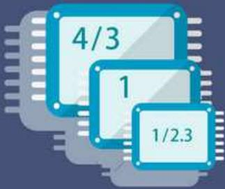
DJI aircraft's camera has a 1/2.3-inch, 1-inch, or 4/3-inch, etc. sensor. The size of a camera sensor refers to the length of the diagonal line of the sensor. A larger sensor indicates a larger signal-noise ratio and more image details.
