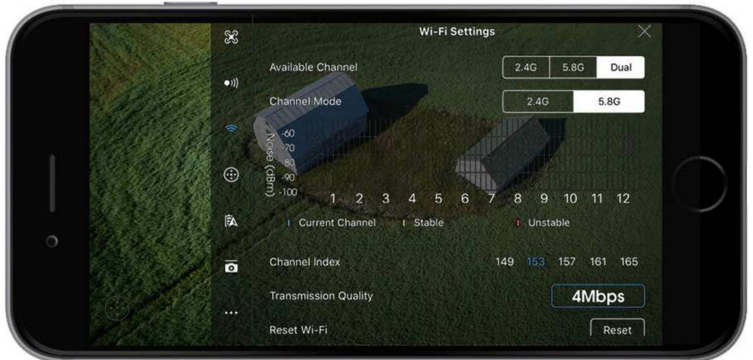
The Wi-Fi settings screen will show you the strength of the Wi-Fi signal, and if there is any interference, also you can use it to switch it from 2.4 GHz to 5.8 GHz. You can also reset the Wi-Fi settings and change the username and password. **(Mavic, Spark only)**
