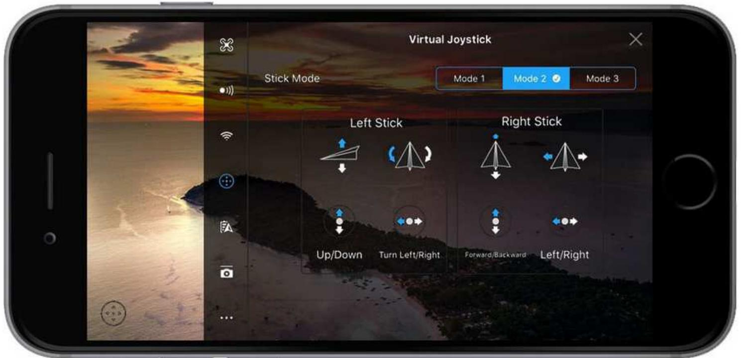
This is where you can choose the stick mode for how to fly your aircraft; the default joystick mode is 2 for both the remote controller and the virtual joysticks. **At present, only the Mavic and Spark support virtual joysticks.**
