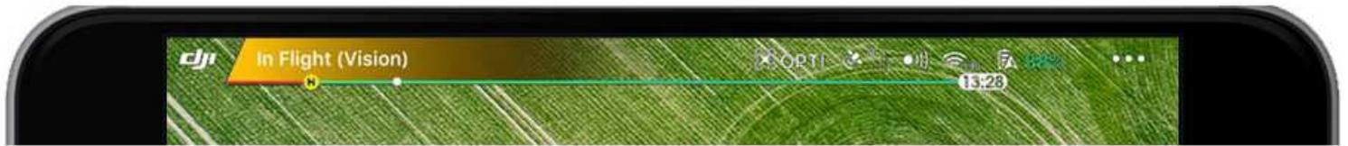
This shows you how much power your battery has left. The line gets shorter as the battery power is depleted. The first dot on the left is when the drone will automatically land due to low power. The second dot is when the app will try to activate RTH unless you stop it. The yellow H represent your home point and moves along the line to show how much power you will need to get your drone back home.
