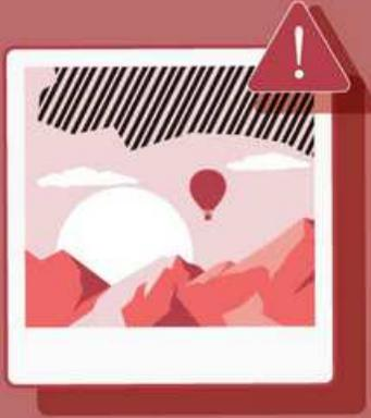
On the preview screen, zebra stripes will be shown over the areas that are overexposed. When the zebra stripes appear, try decreasing the exposure to minimize overexposure in the image. The overexposure zebra stripes warning will not be recorded in the captured image.
