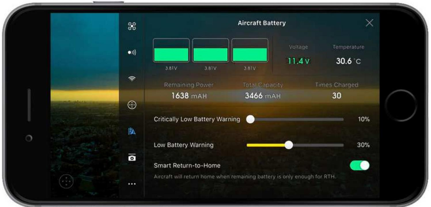
Shows your battery's health. You can adjust Critically Low Battery Warnings and Low Battery Warning percentages here, and this will change when the app sends you a warning about the battery level. Read this article to learn more about your [intelligent battery and how to care for it](#).
