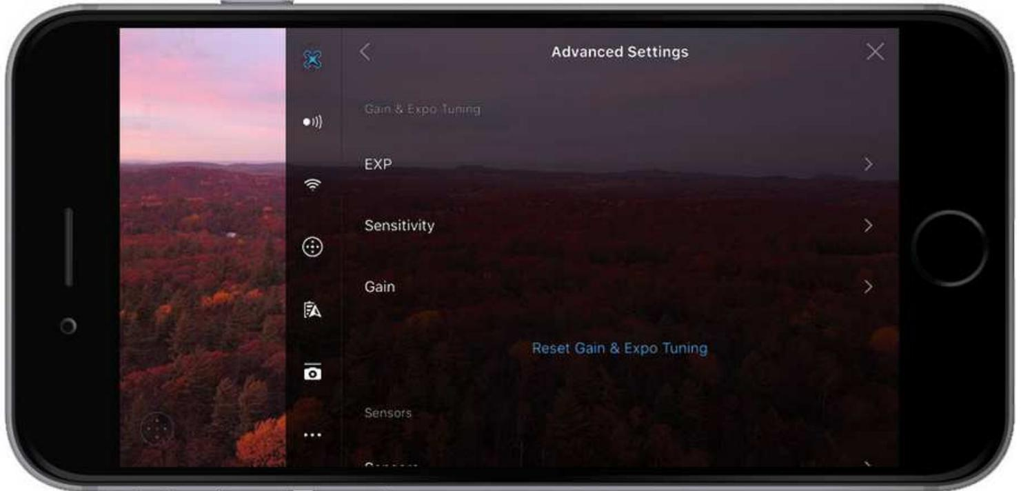
These settings control how fast the stick inputs are translated into movement by the drone. The higher the value, the more responsive the drone will be to stick movements.
