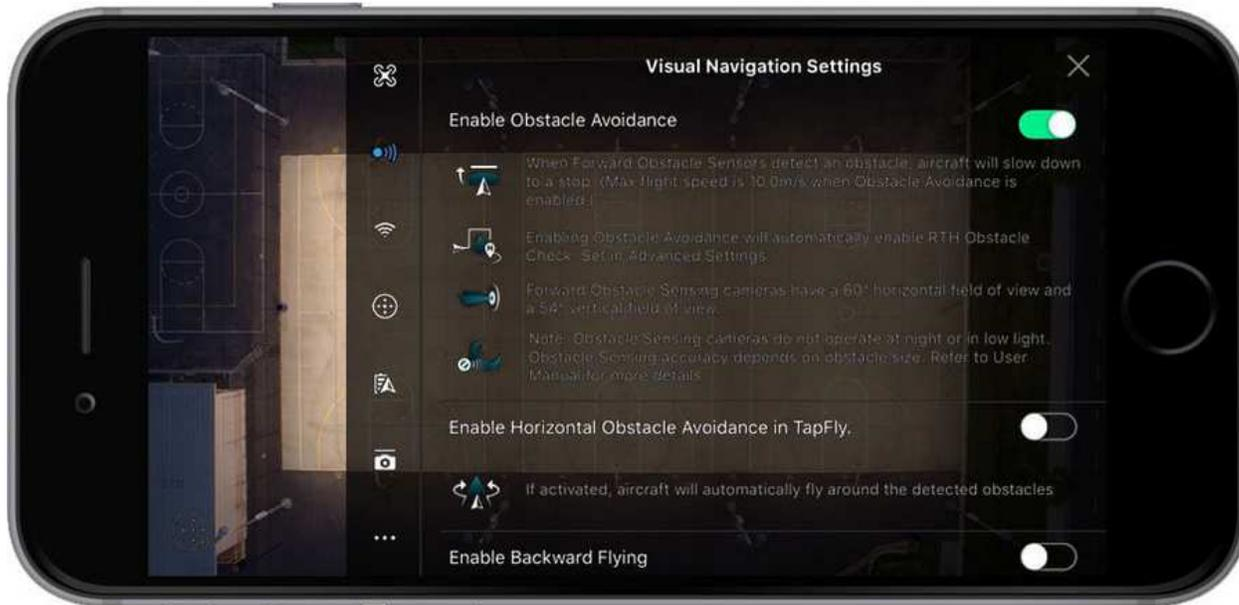
**Enable Obstacle Avoidance:** With this setting enabled your aircraft will detect obstacles in front of it, and it will limit the max speed to 10 m/s, so the aircraft has time to break when it detects something. **Obstacle avoidance may not work in low light situations (300 lux or below), and it will struggle to detect thin obstacles such as wires.**
